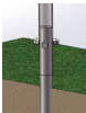
用螺栓锁紧柱子和地钉 Fix the post and ground screw with bolts.
